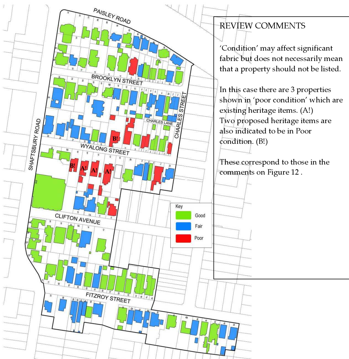
Figure 11 in Study: Diagram showing condition of properties within the Shaftesbury East Study Area. (Note: 10 Wyalong is not visible from the street and therefore no condition is identified for it.)
